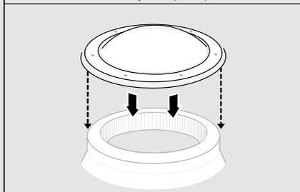
**5** Fix dome to completed upstand using 55mm dome fastener, fastener button, steel & foam washer
