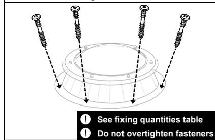
**4** Install roof covering to cover kerb in accordance with manufacturers installation recommendations
