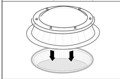
**3** Fit kerb to roof using 55mm kerb fasteners
